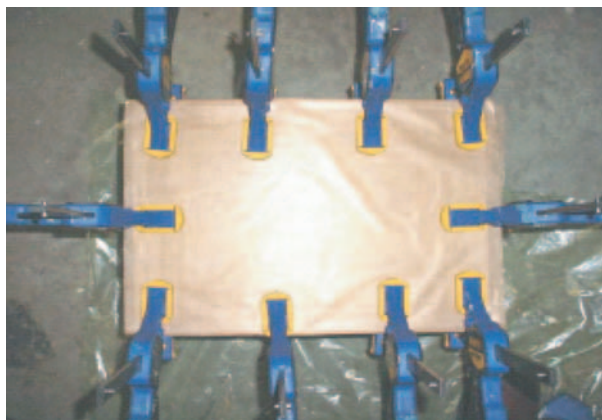
Figure 32. Casting of foam in aluminum mold. (Reprinted from [301] with the permission of SAMPE.)
