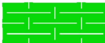
Figure S13. Schematic illustrations of (A) square cut pattern with a unit aspect ratio of 1 and (B) rectangular cut pattern with a unit aspect ratio of 2.5.
