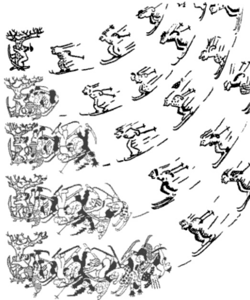
Figure 2. Schematic picture of continuous pushing of shock wave (from Courant and Friedrichs, 1950).
