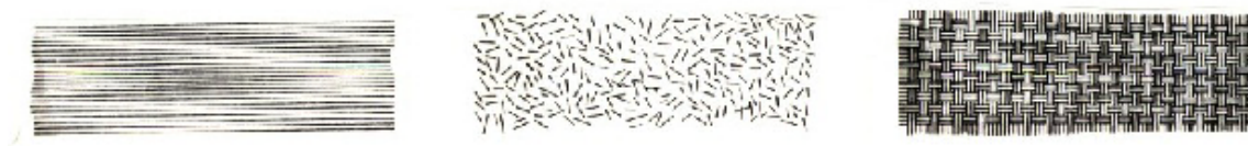
Figure 4 – Schematic Illustration of Fiber Types: Unidirectional, Chopped & Woven. [Shackelford, 1996]
