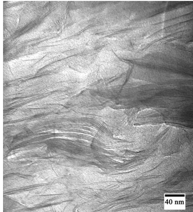
Fig. 6. TEM micrograph of a montmorillonite poly (L-lactic acid) nanocomposite, showing both intercalated and exfoliated states [15]. Reprinted with permission from [15]. Copyright (2003) American Chemical Society.
