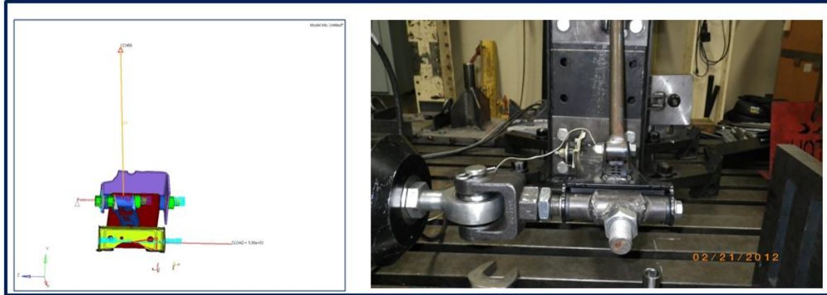
Figure18: Fore-aft Loading FE Model and Test Set up
