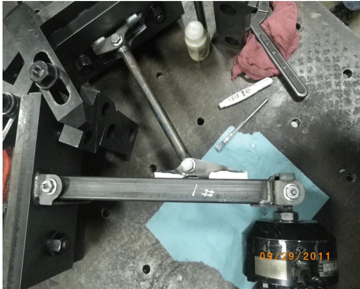
Figure8: Test Set-up of simplified suspension assembly
