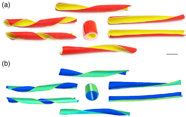
Figure 2. a) A series of different configurations of the neutrally stable structure with the same radius of 42 mm, which can be transformed between configurations in each direction in experiments. b) FEM solid model built in COMSOL5.5 for the estimation of the stress and distortion profile. Bar = 50 mm.
