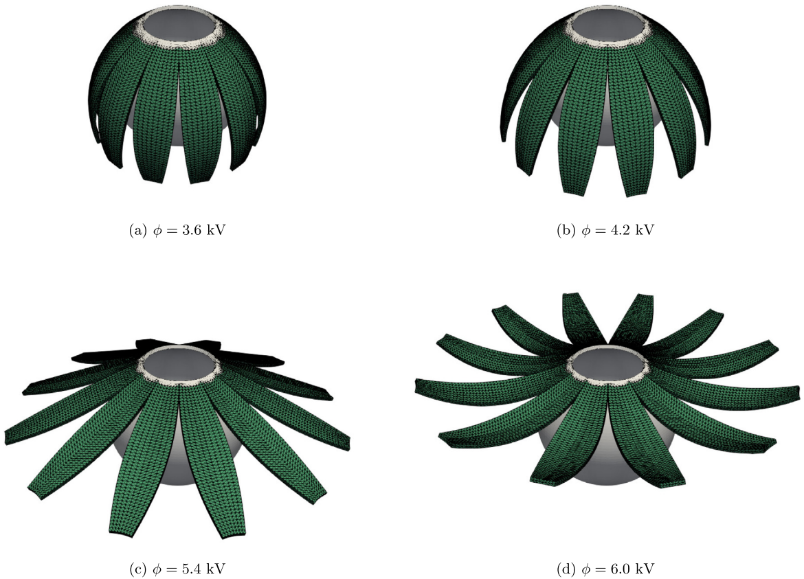
Fig. 14. Spherical gripper: deformed shapes of the gripper at different values of applied voltage.
