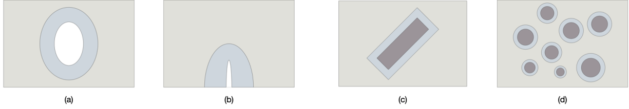
Figure 3: Cloaking of an elliptic hole (a), an elliptic cut (b), a rectangular inhomogeneity (c), and randomly distributed circular inhomogeneities (d). The blue color shows the cloak C .
