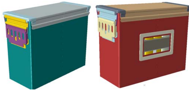
Figure 3. U.S. Army M548 Ammunition Storage Container original and proposed design with vents
