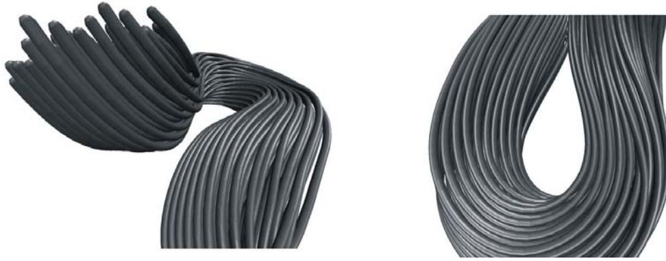
Figure 13: Detailed view of a highly deformed CNT bundle under compressive load.
