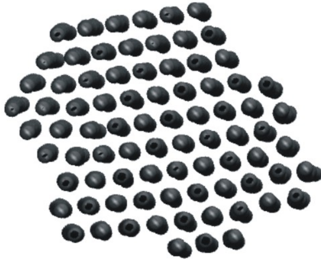
Figure 11: Bundles of CNTs. Cross-sectional view of a bundle of CNTs forming a nanowire, with 81 CNTs. This material forms a two-dimensional hexagonal structure. We note some crystal defects in this case. This also shows the cross-sectional shape of the CNT nanowire. The equilibrium shape features straight surface structures. Some crystal-type defects such as a twin GB exist in the equilibrated structure. Similar structural features have been observed in all-atomistic studies of bundles of CNTs [42].
