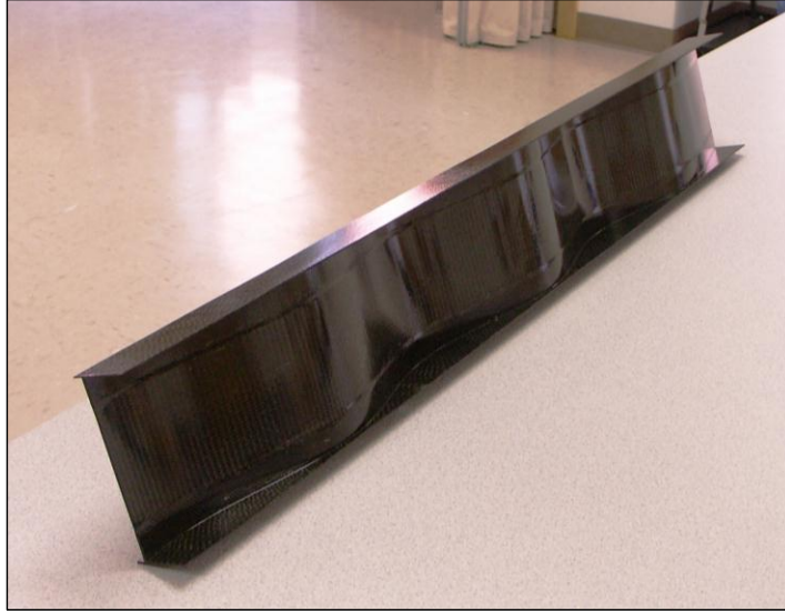
Figure 1. Sine wave beam application with 3D woven composites.
