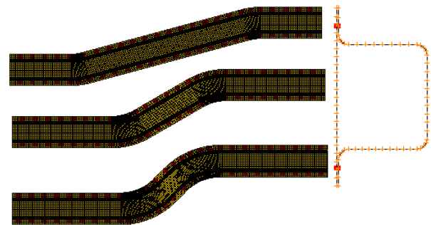
Figure 3: Undeformed model and cross-section for 15°, 30°, and 45° frames. Red dots represent spot weld locations.
