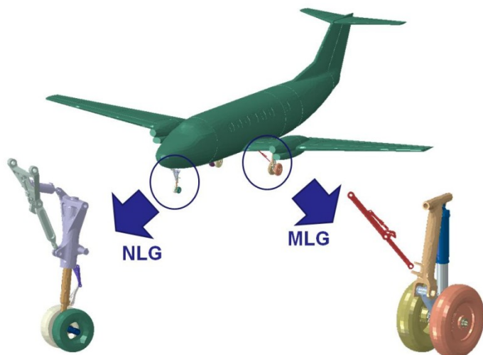
Fig. 1: Aircraft landing gear system
